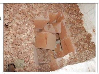
In addition to the compliance and penalty implications, cold face failures can be both expensive and disruptive. It takes a good deal of time to pull out all of the ceramic media, remove the faulty supports, install new supports and reinstall the media. And, during the repair process, the facility has the choice of losing money by shutting down production or risking increased penalties by operating the process uncontrolled.
