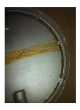
This photo depicts a typical regenerative butterfly valve platter and seat. Over time the seal created between the platter and seat will widen. Reasons for this may be poorly designed valves, condensation build up on the valve, temperature failures, etc... Routine inspection and possible adjustment is necessary to insure a tight tolerance and zero leakage.
