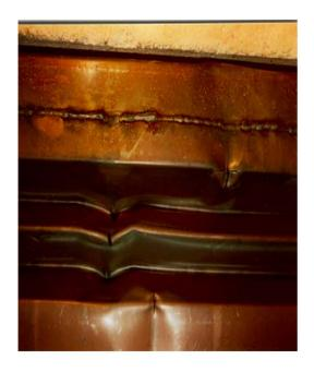
This photo shows failure of a typical shell and tube expansion joint. The tears in the expansion joint are a path for VOCs to escape directly to the exhaust stack, thereby lowering the performance capability of the thermal oxidizer – even though the combustion chamber may be held at the permitted minimum operating temperature.
